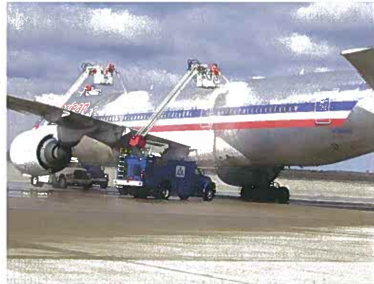
More than 200 gallons of propylene glycol can be used per plane for deicing.
