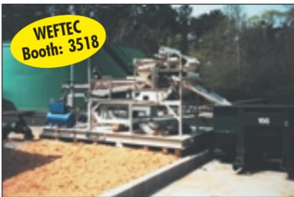
A series of affordable compact belt filter presses and gravity belt thickeners specifically designed for smaller municipal wastewater plants is offered by PHOENIX Process Equipment Co.
