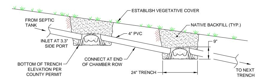
\*NUMBER OF ROWS DETERMINED BY DESIGN AND CENTER TO CENTER SPACING PER CODE.
