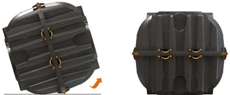
12. Visually inspect the seam to ensure that the gasket remains securely seated within the tank top and bottom half seam grooves. Starting on each of the tank ends, place the open side of a seam clip against the joined seam of the tank halves and fasten as described in step 8. Fasten the remaining seam clips sequentially around the tank; either clockwise or counterclockwise. Fully engage all seam clips as described in step 8.
