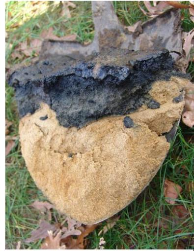
*Figure 6 - Clogged infiltrative surface*
