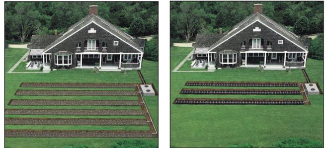
*Traditional full-size stone and pipe leachfield vs. reduced size chamber system leachfield.*
